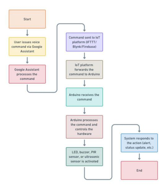
Figure 1. Flowchart of VOXAIOT Voice-Controlled Automation System
